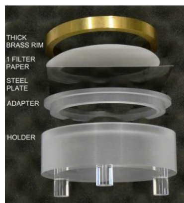
Figure 4 ASTM E2187 stainless steel/filter paper substrate
